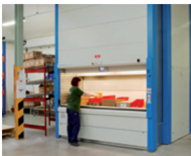
Kardex: automated high-capacity storage system.
